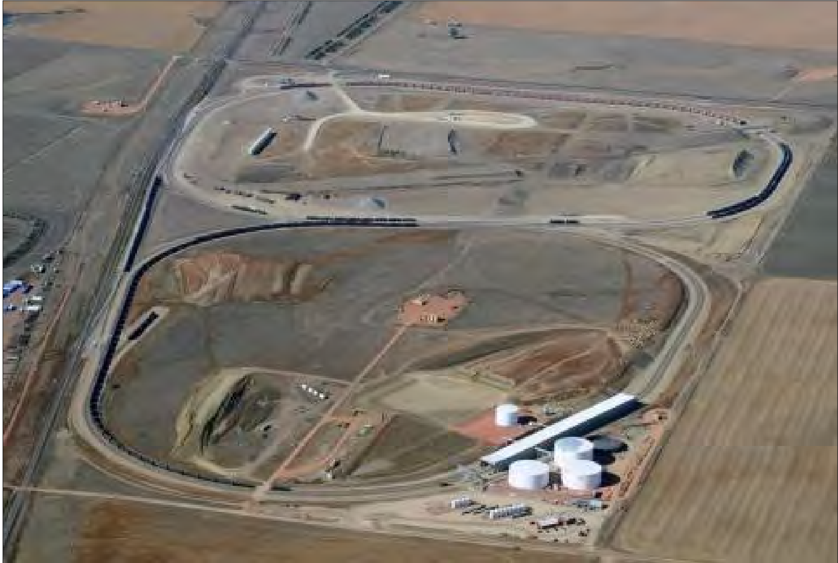
Figure 9-1 Example Crude Oil Rail Loading Terminal
